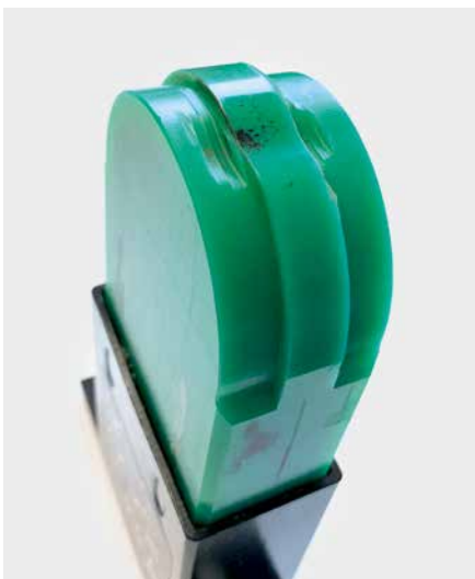
Possible wear pattern due to overloading the Spann-Box®
